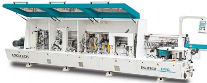
EV583 Series Edge Bander, with Pre Milling, Rough Trimming and Spray Release
